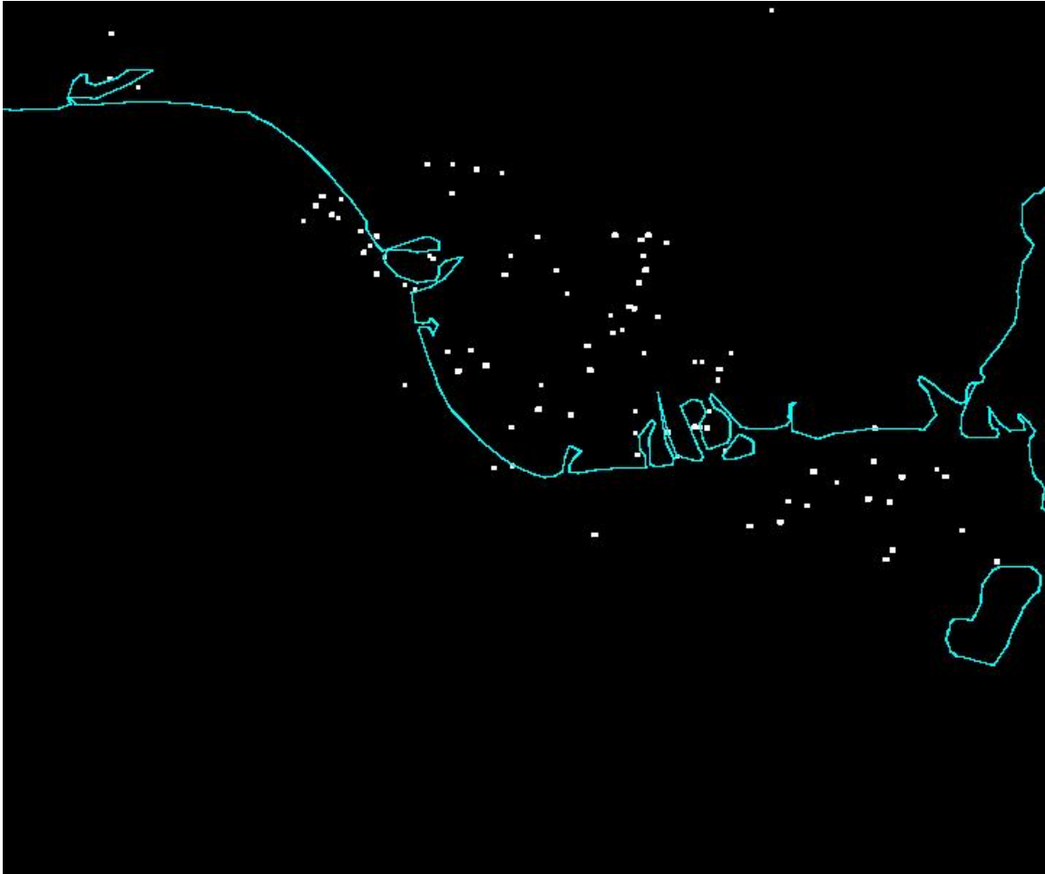
Figure 22. A dilation was applied to the Figure 21 image to generate this mask, which was used to extract the T4mT11 image data of gas flares.
